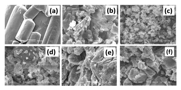
Fig. 1: SEM micrographs of (a) pure Isoniazid, (b) Co(II)-INH, (c)Cu(II)-INH, (d) Fe(II)-INH (e) Ni(II)-INH (f) Fe (III)-INH complex particles.
